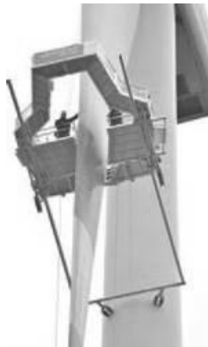
Figure 1: Conventional climbing frame for WTB [2]
